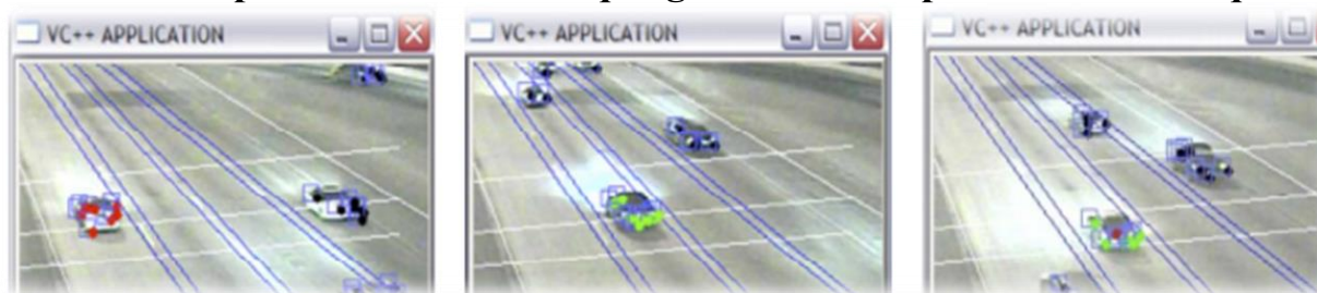
(a) (b) (c) 3-rasm. Turli yo'laklardagi transport vositalarida Harris-Stephen burchak nuqtalarining aniqlanganligi.
