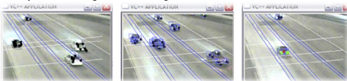
(a) (b) (c) 2-rasm. Transport vositalarida aniqlangan Xarris-Stephen burchak nuqtalari.
